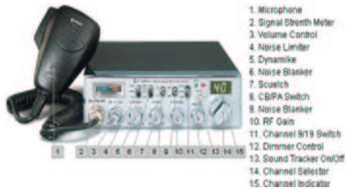
**Fig. 3.** A technical drawing of a cb radio. Leaders are *s*-type and the labels are treated as legends.
